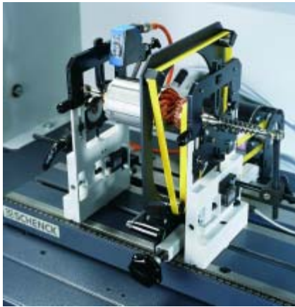
Balancing machine type HM10 with overslung belt drive
