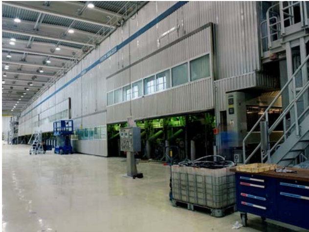
Picture 1: Drying section in a paper mill. Because of the housing in this part of the machine, the use of optical measurement methods is limited. Rolls above or below the drying cylinders can only be measured with additional optical equipment like mirrors or prisms. Such additional equipment reduces the accuracy of the measurement seriously.
