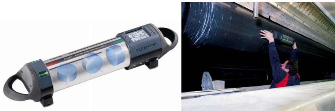
Picture 2: On the left, the measurement device PARALIGN with the ring laser gyroscopes in blue. Each gyroscope measures the angle of its rotation axis shown in red. Unlike traditional systems, no line of sight to the rolls from outside the machine is needed. In the right picture the use of PARALIGN is shown. The device is placed on the surface of the roll; afterwards the roll's position is measured by moving the device along the roll.
