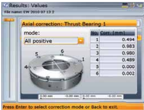
Thrust bearing correction screen
