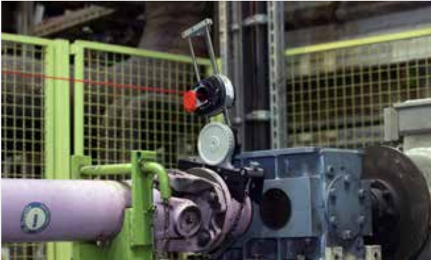
Rotating arm bracket for restricted rotation areas.
