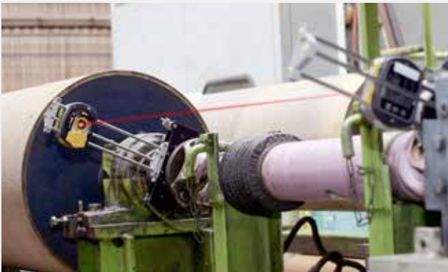
Bracket set for 180° rotation requires only two readings.
