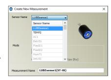
For ultrasound measurements, UAS3 gives you the option to choose either Static or Dynamic and for temperature measurements you can set the measurement interval and the emissivity.
