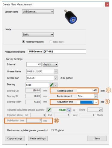
Press "SAVE" and all settings for the selected asset are ready. These settings are assigned to the selected asset and go with it when workorders are transferred to the LUBExpert instrument. No further settings need to be done (nor can be done) in LUBExpert once in the field. This enables your grease technician to have comfortable, fast, and safe work in the field, as well as tight work control and dependable data for the Lubrication Manager.
