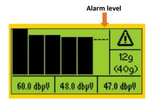
FREE MODE lets you decide on each step you want to take and provides on screen details about the signal development. NOTE that FREE MODE will not guide you with recommendation for the next step and status and will not stop you with conclusion that the task is finished. However, FREE MODE will deliver a final conclusion about the lubrication process to UAS3
