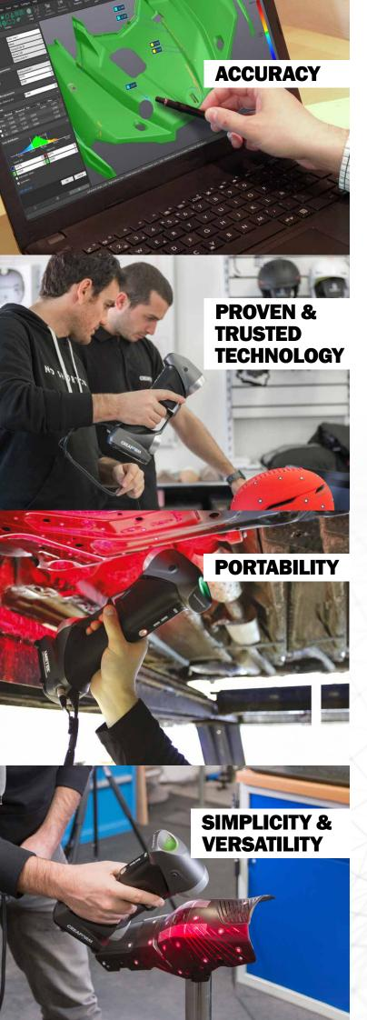
The HandySCAN 3D | SILVER Series delivers accurate and reliable 3D measurements regardless of the measurement setup quality and the user's experience level. Featuring dynamic referencing, both the scanner and part can move freely during scanning, and an accurate and high quality scan can still be obtained.
