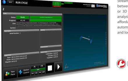
Streamline software provides a clean integraton between the Universal Robots' cobot, the selected 2D or 3D sensor, and PolyWorks to automate the data analysis and reporting. 3D Infotech is able to deliver an affordable, flexible, mobile and easy-to-use automated inspection solution capable of both global and local measurements.
