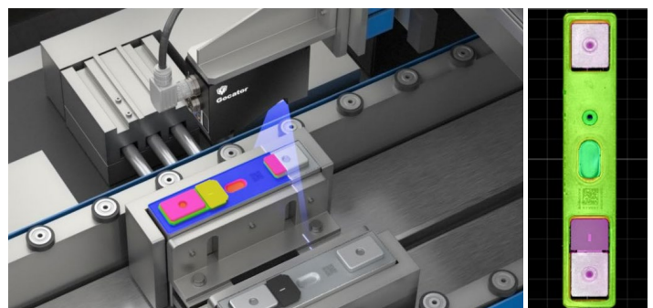
EV Battery Module Inspection with Gocator 2640
